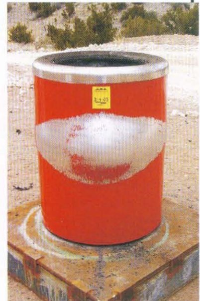
Post-detonation Picture: "This is a close-up post detonation photo, from a side wall test using C4 explosives"
