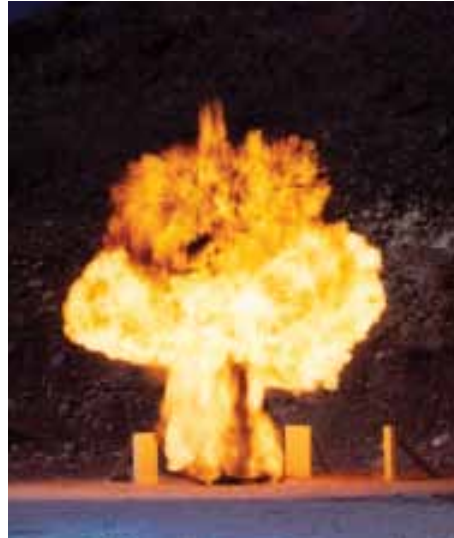
Side wall test photo taken at EMRTC of a bomb resistant trash receptacle using C4 Explosives.
