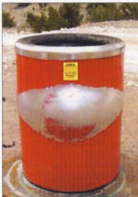
This is a close-up post-detonation photo, from a side wall test, using C4 explosives.
